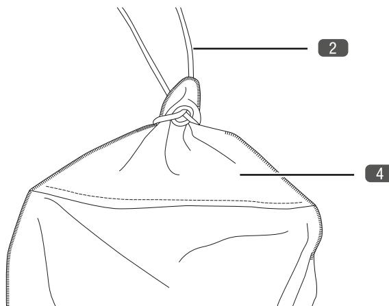
2. Open the fastener on each of the four anchor bags and fill the anchor bags with plenty of damp sand to ensure the ballasting and stability of the product.
