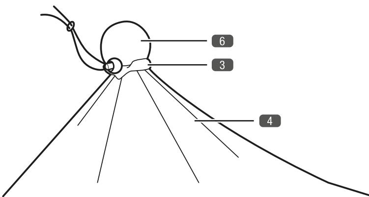
2. When you are satisfied with the position of the product, secure each anchor bag with a ground anchor 5. Insert the ground anchor through the loop on the anchor bag and then into the ground as far as it will go (see Fig. 6). Make sure once again that the lines are taut.
