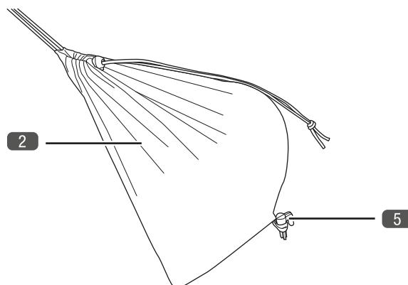
**i** The lines on the anchor bags 2 can be shortened as required during use by pulling the lines through the anchor bags and fastening them with the fastener.
